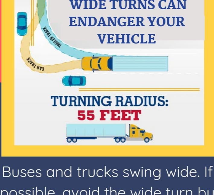
possible, avoid the wide turn by positioning your vehicle outside the turning radius.
